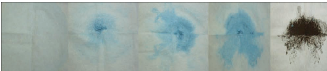
Fig. 9. Images of filtration sheets of dye solutions prepared in medium without ultrasound at 5 different pH (pH 1–4–7–10–13) at 6 g/L dye concentration with 1 g/L dispersing agent
