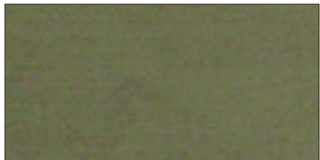
Fig. 14. Wool fabric dyed with copper naphthenate compound
