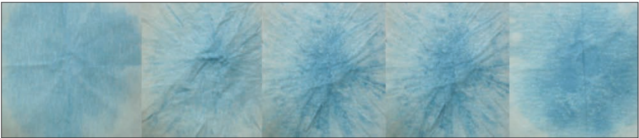
Fig. 12. Images of filtration sheets of dye solutions prepared in medium with ultrasound at 5 different dye concentrations (2–4–6–8–10 g/L) at pH 7 with 1 g/L dispersing agent
