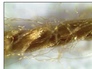
Fig. 8. Upper thread 150 tex PES/PES, coded as thread 3, used in fabric C, at 1 000 rpm
