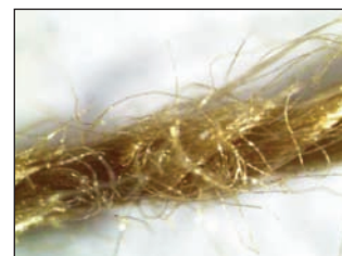
Fig. 10. Upper thread 150 tex PES/PES, coded as thread 1, used in fabric C, at 2 000 rpm
