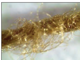
Fig. 14. Upper thread 150 tex PES/PES, coded as thread 3, used in fabric C, at 3 000 rpm
