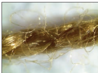
Fig. 11. Lower thread 150 tex PES/PES, coded as thread 3, used in fabric C, at 2 000 rpm
