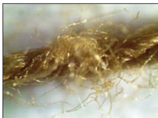
Fig. 12. Upper thread 150 tex PES/PES, coded as thread 1, used in fabric B, at 3 000 rpm
