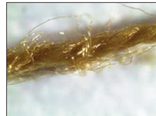
Fig. 6. Upper thread 60 tex PES/PES, coded as thread 1, used in fabric C, at 1 000 rpm
