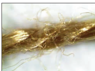
Fig. 13. Lower thread 150 tex PES/PES, coded as thread 1, used in fabric B, at 3 000 rpm
