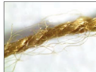
Fig. 7. Lower thread 60 tex PES/PES, coded as thread 1, used in fabric C, at 1 000 rpm
