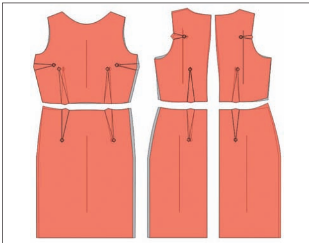
Fig. 16. Comparison between basic dress pattern design for the normal (grey) and scoliotic female (red)
