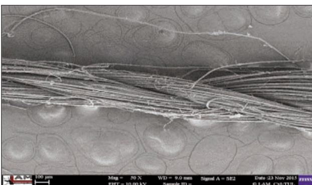
Fig. 7. SEM image of sample 2A before sewing
