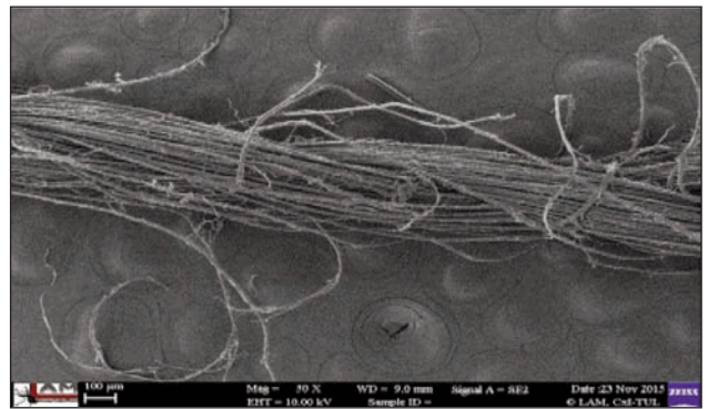
Fig. 4. SEM image of sample 1A after sewing (4000 r/min)
