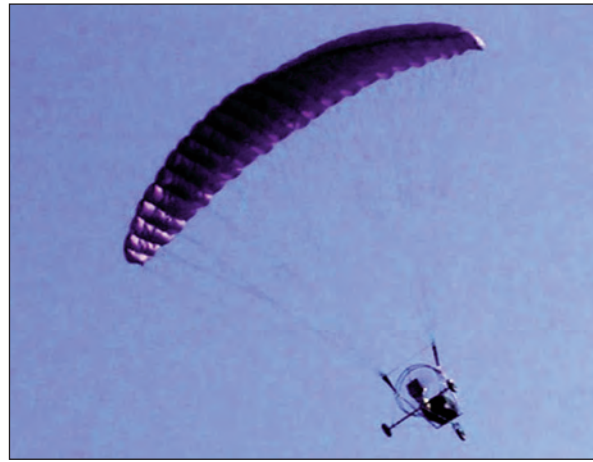
Fig. 6: Parachute in remote controlled flight
