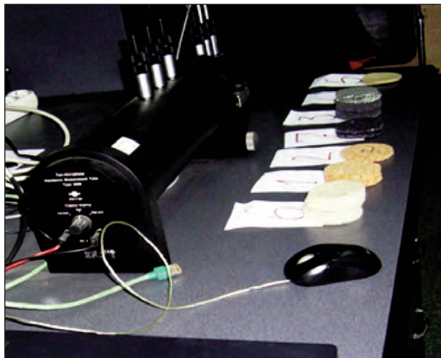
Fig. 1. Tube type 4206 A for impedance reading
