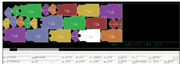
b – Marker plan prepared according to the 2 nd fabric
