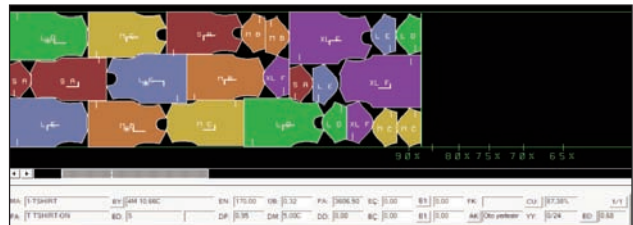
a – Marker plan prepared according to the 1 st fabric
