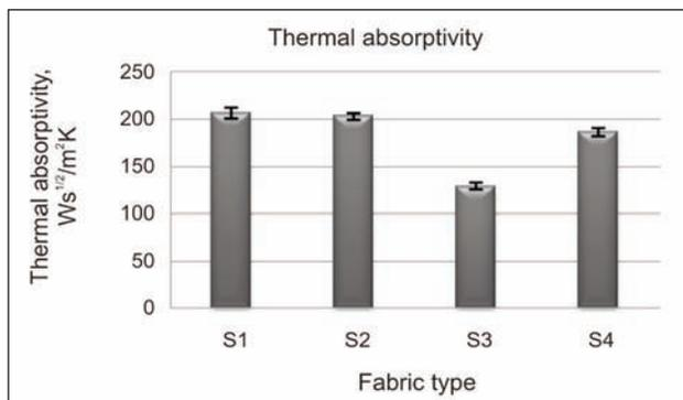
Fig. 8. Thermal absorptivity of the tested fabric samples
