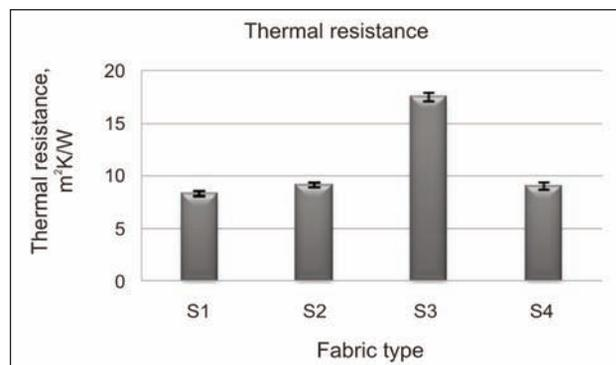
Fig. 9. Thermal resistance of the tested fabric samples
