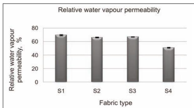
Fig. 10. Relative watervaporpermeability of the tested fabric samples
