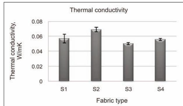
Fig. 7. Thermal conductivity of the tested fabric samples
