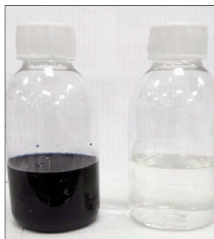
Fig. 11. Aqueous dye solution containing Indigo dye (left), water treated with ELM Process (right)
