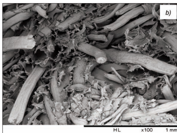
Fig. 1. SEM micrographs of fracture surfaces associated to composites with (a) raw and (b) treated Posidonia fibers
