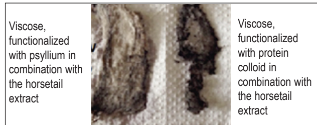
Fig. 2. Biodegradability of functionalized viscose samples after seven days of burial in the soil
