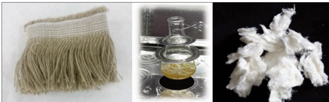
Fig. 1. Waste jute fibers, pulping process and recycled cellulose
