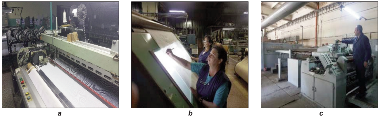
Fig. 1. Aspects from the weaving operations (a), quality control (b) and finishing (c) of functional models development of the woven structures with controllable permeability meant for the canopy of the stabilization-deceleration system
