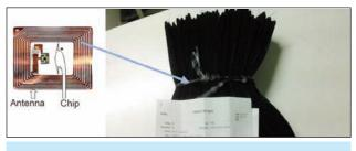
Fig. 3. Batch with RFID tag
