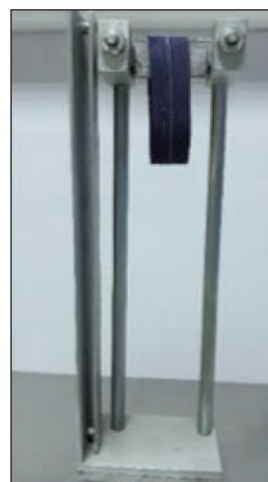
Fig. 4. Heart loop test apparatus and sample placement
