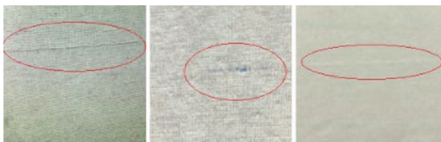
Fig. 2. Defects commonly found in recycled fabrics: a – half-width weft; b – fiber in color; c – thin thick weft
