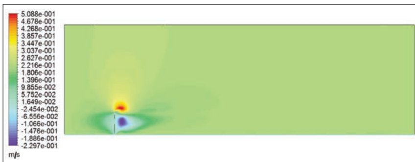
Fig. 4. The contour for the velocity field on x direction, for barrier porosity p=64\%
