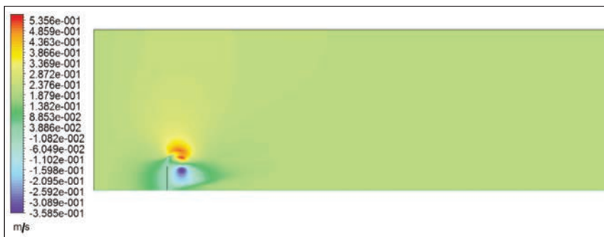
Fig. 3. The contour for the velocity field on x direction, for barrier porosity p=0\%
