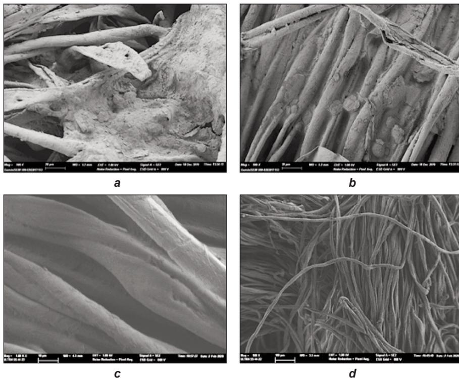
Fig. 9. SEM images of: *a* – untreated fabric, sample 1 at 500×; *b* – untreated fabric, sample 2 at 500×; *c* – treated fabric, sample 1; *d* – treated fabric, sample 2 at different magnifications ×1000, ×500 and ×100
