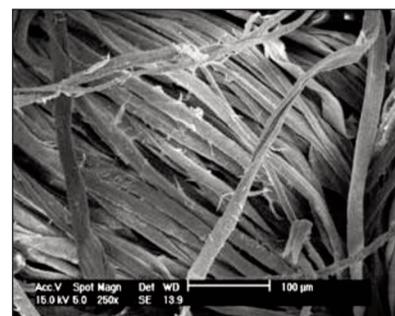
Fig. 4. SEM image of the fibres form traditional shirt “ie”, from Hateg County at 250 $\times$  magnification
