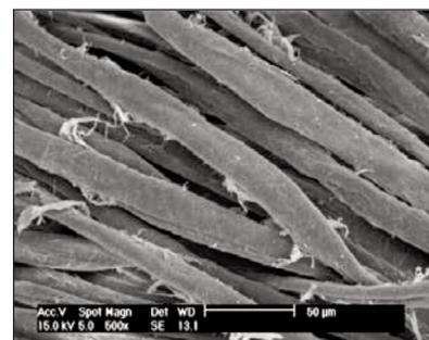
Fig. 6. SEM image of the fibres form traditional shirt “ie”, from Hateg County, at 500 $\times$  magnification
