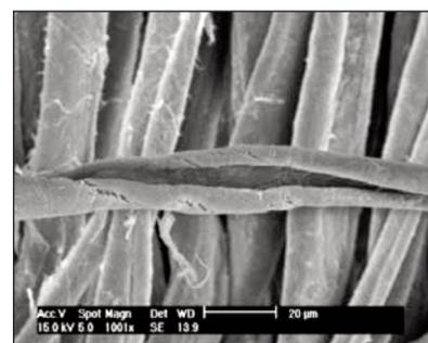
Fig. 8. SEM image of the fibres form traditional shirt “ie”, from Hateg County, at 1000 $\times$  magnification
