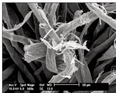
Fig. 5. SEM image of the fibres form traditional shirt “ie”, from Hateg County, at 500 $\times$  magnification
