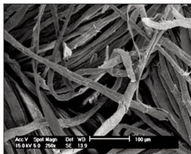
Fig. 3. SEM image of the fibres form traditional shirt “ie” from Hateg County, at 250 $\times$  magnification
