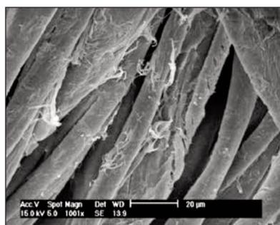
Fig. 7. SEM image of the fibres form traditional shirt “ie”, from Hateg County at 1000 $\times$  magnification
