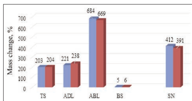
Fig. 6. Mass changes of samples: ■ wet bending samples; ■ wet compressed samples
