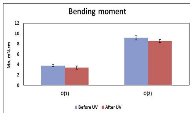
Fig. 9. Bending resistance moment values before and after UV
