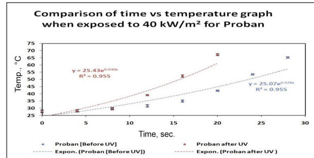
Fig. 7. Time vs temperature graph when exposed to UV for specimen B before and after UV exposure
