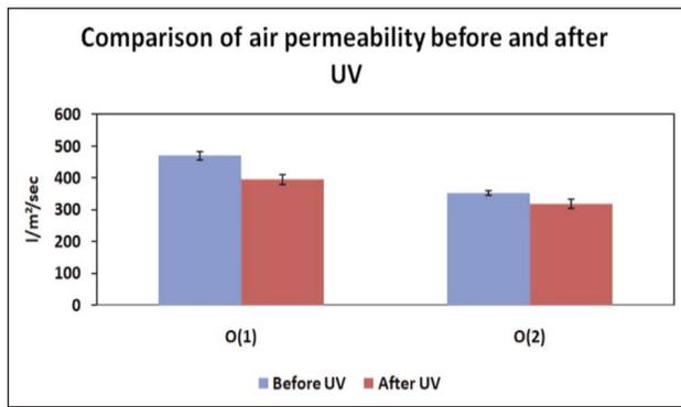
Fig. 5. Air permeability values before and after exposure to UV
