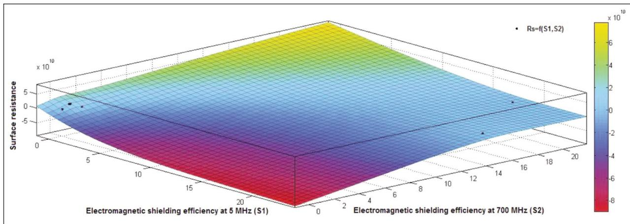
Fig. 10. 3D representation of the surface resistance ( $R_s$ ) according to the electromagnetic shielding efficiency at 5 MHz ( $S_1$ ) and electromagnetic shielding efficiency at 700 MHz ( $S_2$ ),  $R_s = f(S_1, S_2)$
