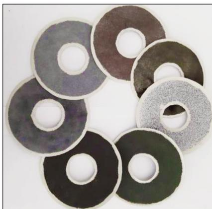
Fig. 2. Ag-contoured samples to measure the effectiveness of electromagnetic attenuation
