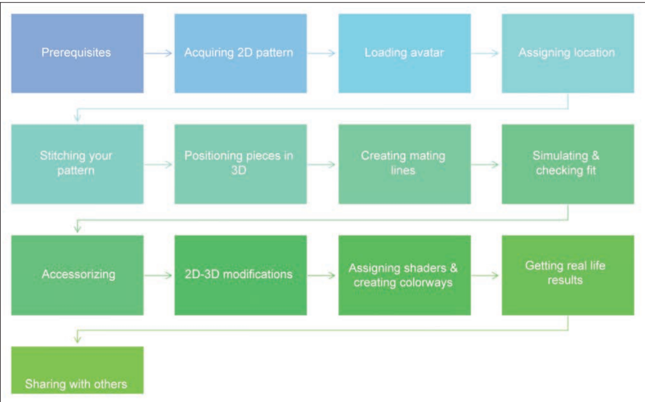
Fig. 1. Workflow for transforming into 3D samples of EM01–EM014
