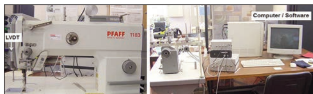
Fig. 1. The control device in the lockstitch sewing machine and connected PC
