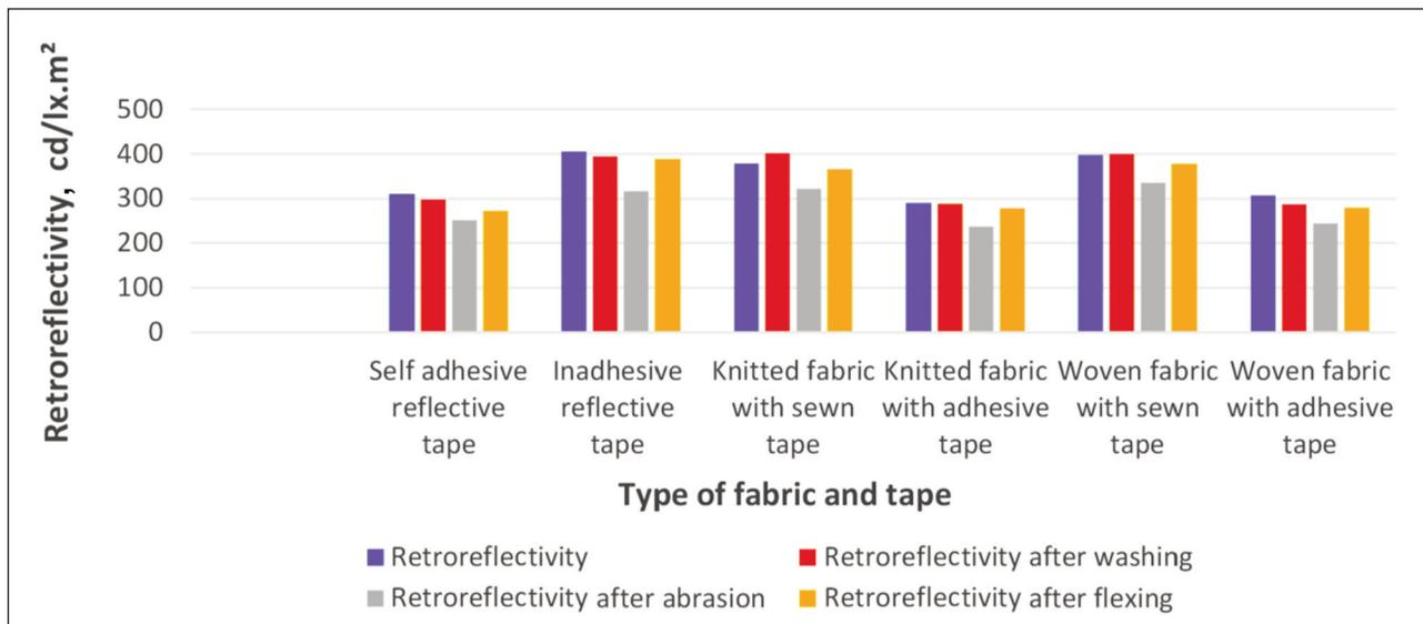
Fig. 3. Retroreflective performances of samples after various effects
