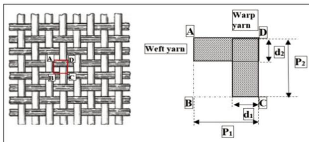
Fig. 1. Diagram of the weave structure
