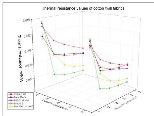
Fig. 3. Comparison of predicted and observed resistance values of cotton fabrics with: a – plain; b – twill
