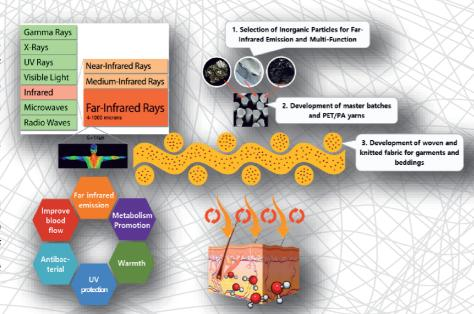
MAIN RESULTS: Technology to prepare highly efficient far infrared and anions release nanocomposites; innovative method to uniformly disperse the nanoparticles into final yarns and preserve their genuine properties; Development of pyroelectric/multifunctional fabrics mainly based on natural yarns (cotton, bamboo).
